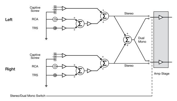
Figure 7. MPA 152 Plus Summing Diagram
